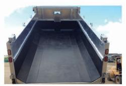
From start to finish, Avalanche dump truck liners are produced in house. We produce the sheet, butt-weld the plastic liner, and complete the custom fabrication all in the same facility.
